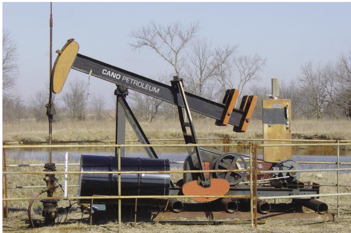
With oil and gas prices at record highs, producers are having little difficulty in finding financing to help grow their business through conventional bank debt and other means. This pumping unit is on a stripper well operated by Cano Petroleum in Nowata County, Okla.
